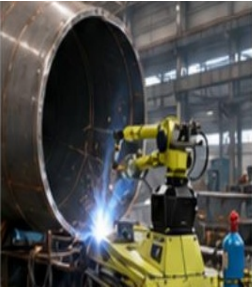
3 Heavy vessel welding
